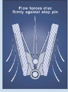
**DISC SEAL OVERLAP:** Contact between the seal and the disc is uniquely designed to eliminate indentation ridges found in designs
