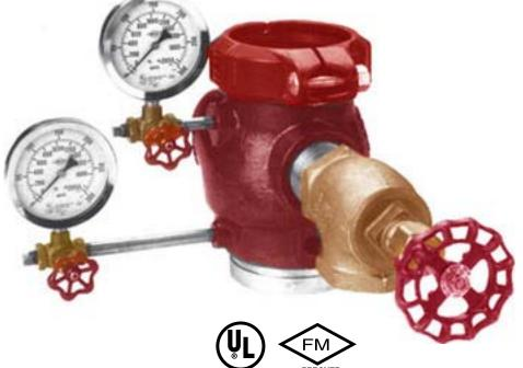
The 2<sup>1</sup>/<sub>2</sub>"to 8" Grooved End Riser Check Valves are designed and intended for use in a wet-type automatic sprinkler system. It reduces the possibility of false alarms by trapping a portion of transient surges in supply pressure within the system, thus, reducing the possibility of subsequent surges actuating the Flow detector and its associated alarms.
